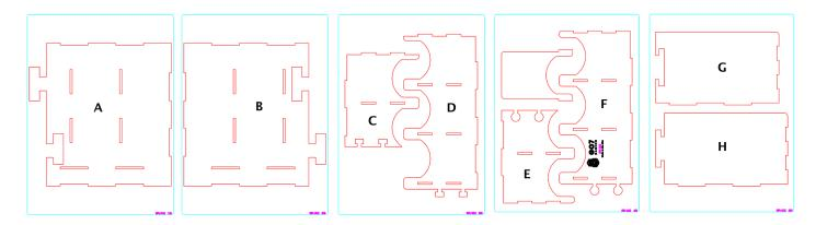
Please reference the diagrams to understand how each component fits together. Also, dry fit the pieces to understand how it goes together and ensure everything is oriented properly before applying glue. Finally, cleanup excess glue to ensure a proper fit and finish, especially in card, rail, and tray storage areas.
