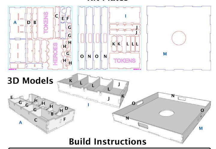
Finally, let's build the last few trays! After each piece is placed, you should cleanup excess glue using the provided glue sticks (short, thin wood strips). Also, remember to dry fit everything so you understand where to place glue and how everything fits together.
